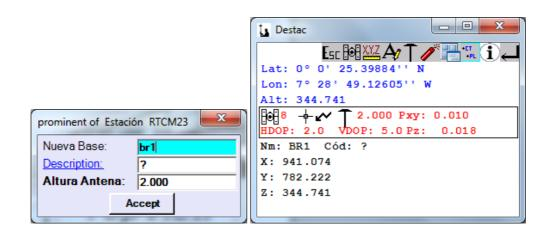
Next, if we have configured the program to get more than one range of readings, we are given the option to save the file, as shown:
