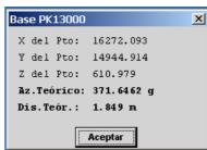
After taking a reading from the device the program informs us of the point with respect to the alignment with the base and the actions to take.
