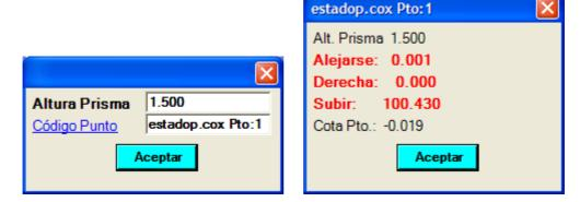
The action "Zoom In" can change to "Zoom Out" if the difference in distance is negative. The 'Right' action can be changed to "Left" and reflects the lack of alignment in the stakeout. The action Up may change to Down depending on the difference between the real height and the height to be staked.
