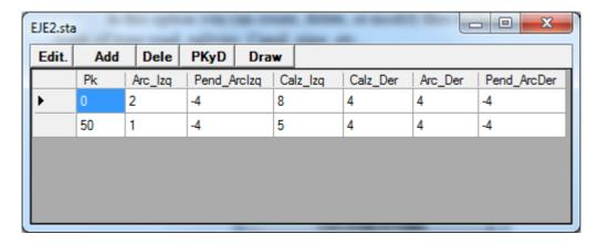
On the road shoulders you can specify a slope for the item which will be applied provided that the cant is less than this. Walkways will have the resulting slope of the interpolated cambers table applied.
