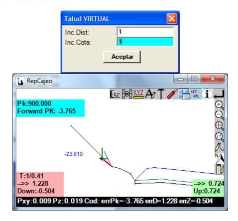
In this example we have defined a vertor 1/1 that starts at the ditch and is more sloped than the original (1/0.5), if we move until the data at the bottom right is ZERO we are at the intersection of the Virtual Slope and the ground.
