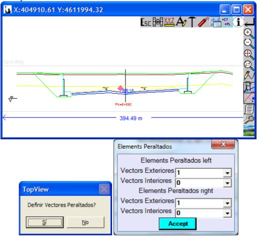
After defining the axis entity and the entity which defines the reference coordinates position, we are asked to select the lines that define the surface of the section and if we want to define camber vectors within those entities we can click on each side of the first cambered section. In this last window we specify how many vectored sections will be influenced by the camber table.
