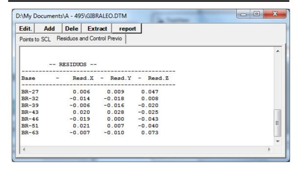
In the Tab "Result and Previous Control" we are shown a previous control of the data in which there is no calculation, but can serve to detect if we have made a mistake when typing the local coordinates, or the geographical coordinates from the GPS. The process is based on comparing the relative differences that exist in distance and increased height between the local coordinates and the GSP. The final part shows the "Spare" calculation results.
