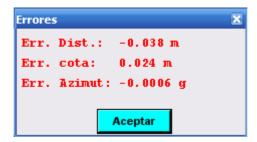
If we choose to just position the equipment, the program will impose an azimuth to the station, and with the third option we include the previous two, ie, connect to another base, read it and obtain the relative errors for distance, elevation and azimuth.
