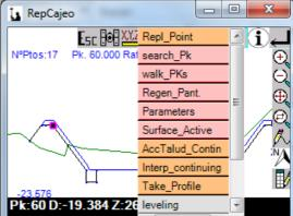
With cursors, we can move through all the points of the layout surface and when we have overcome the last point automatically move on to the next profile. We can do Zoom +-, settings with the pointer, etc..
