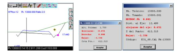
Afterwards, a cross shows the position of the projected point on the profile. Pressing a key displays the actual position of the point and the actions to be taken to position it correctly.
