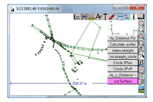
This allows us to perform multiple common computations extracting the coordinates from the points chosen on the screen and the results can be stored in the current file. The coordinates of the selected points can be edited and changed before the final calculation without altering the base.
