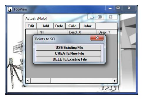
The calculation button creates a file with "Points for SCL" which consists of a register for each Base used for the SCL that has the base name, the Local Cartesian coordinates and the Cartesian coordinates taken by the GPS according to Datum, timezone, and the geoid used for the calculation. This file has the extension \*.dtm and in TopView is shown thus:
