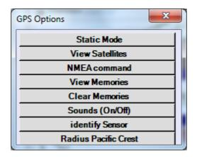
**1.-Static Mode:** In this section we can activate and stop the recording of observations in the internal memory of the receiver and then to perform post-processing. This operation is possible both in the GPS-Mobile and the GPS-Base, although GPS-base is not necessary because because the setting activates parallel recording of observations while resolving ambiguities in realtime (RTK).
