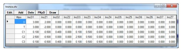
If a name of a family of vectors for gutter is called "C1 v of..." can be called from the table of EMBANKMENTS and DITCHES as "C1 \*", i.e. we can use wildcards for short calls to names.
