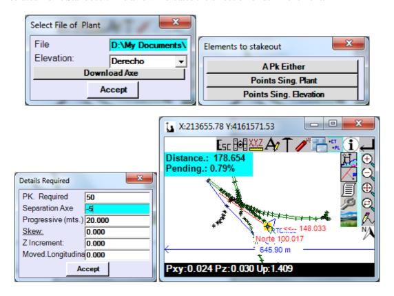
In "**Perp to Axis**" after loading, the program draws the normal from our position to the axis indicating the Pk and calculated displacements. The arrow indicates the direction of our movement.
