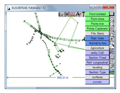
"Isolated point" option allows to stakeout any point. The point can be clicked on screen or be inserted from the list of coordinates. We can either choose, by clicking the icon, entering a stakeout to the north, to the point or base. We can also increase the height of the target point.
