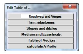
There are elements that are defined parametrically and others vectorially. All ditches, cut and fill slopes (including berms, clearance berms, crowns, etc.), Inadequate fixed platforms (i.e., car parks, pavements, etc.), and inadequate fixed sub-grade (i.e., different thicknesses under areas of parking, pavements, etc...) are defined vectorially. All others are defined as parameters.
