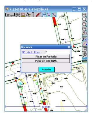
In "File Bases" the program requests the loading of a Bases file and runs a Zoom Extension to display them all onscreen. Afterwards we are asked to select the bases that we want to stakeout and from now on it behaves as in "Isolated Point Stakeout". The drawing of the base differs from the working points in that the crosses are bigger and have a box in the centre.
