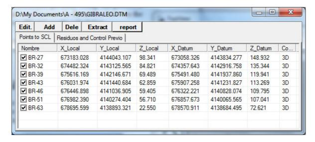
When entering a new "SCL Points" file, the table is empty and to fill it we can go to "Extract" button which requests a file of Bases XYZ (\*.bas) and a Geographic Bases file (\*.lla) where it looks for records with the same base name and places as those in the table. By clicking on "Control" we can switch between "3D", "2D" and "Z".
