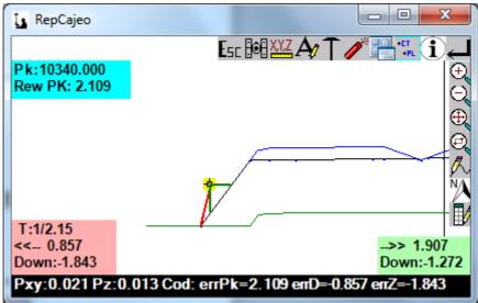
The image at the top shows the stakeout of a 1 meter recess towards the outside point following the slope of the previous item, and without any increase in additional height. The red line shows the way to continue from our position and the position of the point we want to stakeout.
