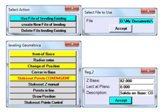
With this module we avoid using a leveling book as all readings (Read forward, Read back) are recorded in a file. Also the dimensions of the bases which are used are read from the same files that we use with ET or GPS, along with the points to stakeout, and are extracted from the COX / CAD file
