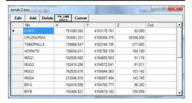
Where we can perform all the actions that appear in the header of each column. The Pk\_Dist option allows you to analyze any base with respect to an axis. The Conver options (PC version) allows calculation of a geographical basis taking into account the chosen SCL and Datum. The result is expressed in WGS84 geographical.
