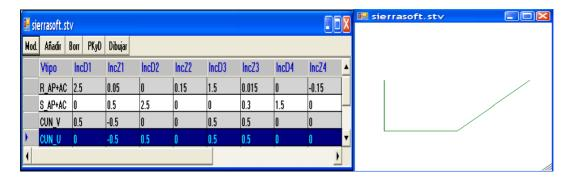
In these images we see two different types of gutters, one V-shaped and one in form of U. We can check as the program operates when it comes to interpolate two families of vectors using the option consult a Pk. The Program will not request a Pk of application for each family of vectors, and a Pk to check the result of the interpolation:
