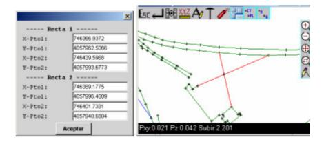
Special attention goes to to "cut surface" that allows a transversal cut on all visible lines on the screen (active layers) and draws that cut..
