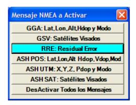
This option allows the activation/deactivation of the emission of different NMEA messages via the serial port of the sensor.-
