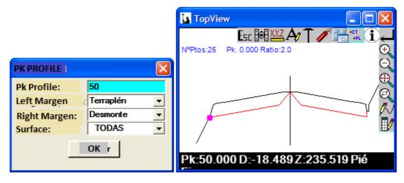
In this graphical display we can move through the points that make it showing at the top data about this point such as distance to axis, the dimension, the element that defines it, and the slope.
