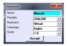
The "Scale" option only appears in the PC version allowing you to scale all program windows for better viewing on high resolution equipment.
