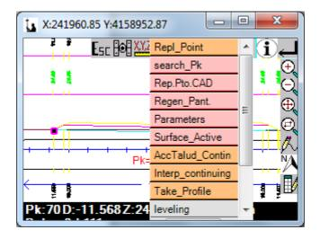
... with the only difference that the second option is "CAD Point Stakeout" that allows you to choose any CAD entity and stake it out in this environment. It is useful if we have elements such as retaining walls, footings, pipes, drains, etc ...
