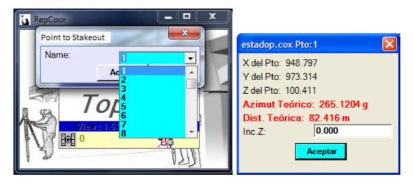
After placing the apparatus with the indicated azimuth and the linear operator, we can check it by pressing Enter. After taking the reading, the program asks for the height of the pole and the code we want to use for the point to save in the backup file.
