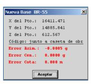
It should be noted that for greater accuracy of the data from the new base, two readings (direct and reverse) are taken.
