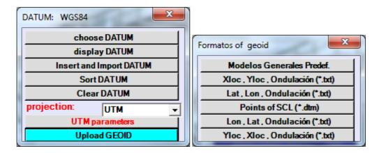
The "Upload Geoid" option has been incorporated with which we apply a model of increments relative to the ellipsoidal bounds obtained directly by the GPS to approach the geoid limit in the area.
