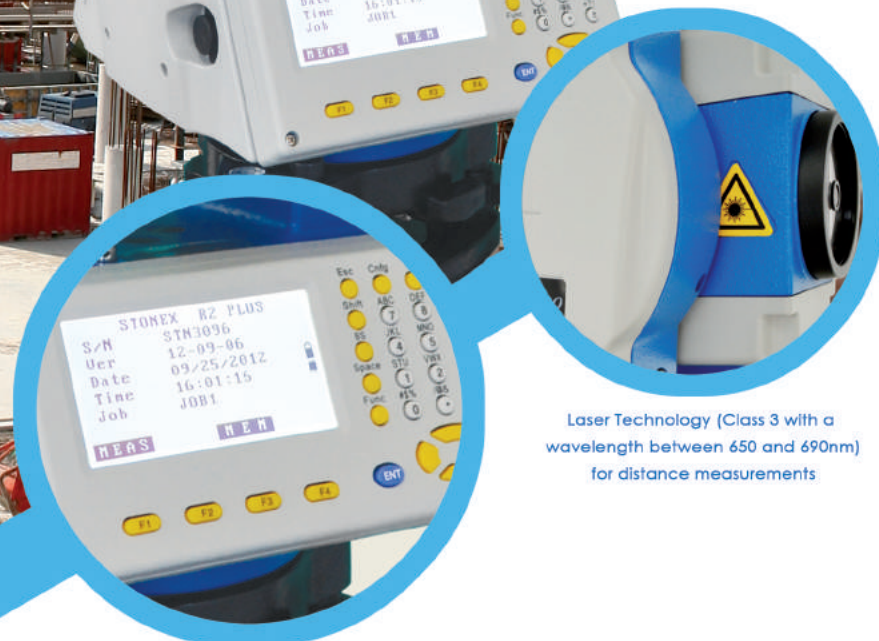
Alphanumeric keyboard on both sides with high resolution backlit large LCD display
